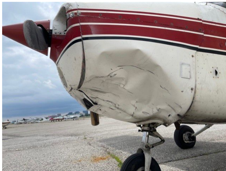
Figure 1: Canadian Flyer 172 damaged by Police drone
